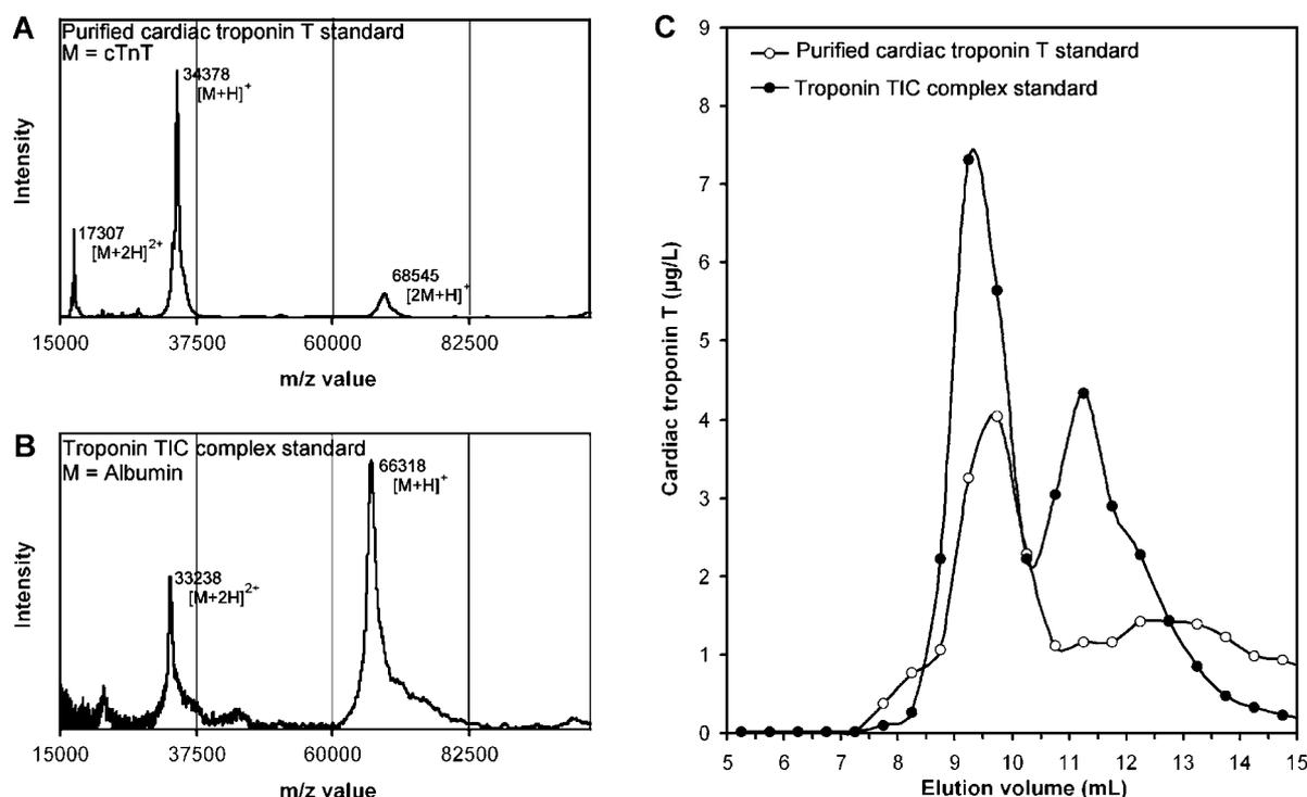
**Figure 2** Characterisation of two cardiac troponin standards. (A) Mass spectrum of a purified cTnT standard showing intact protonated cTnT at  $m/z$  34,378 ( $[M+H]^+$ ). (B) Mass spectrum of a troponin TIC complex standard showing albumin at  $m/z$  66,318 ( $[M+H]^+$ ) as the major component. (C) Elution profile of both cardiac troponin standards spiked into serum and applied directly to SEC. cTnT was measured with the third-generation Roche cTnT immunoassay.
