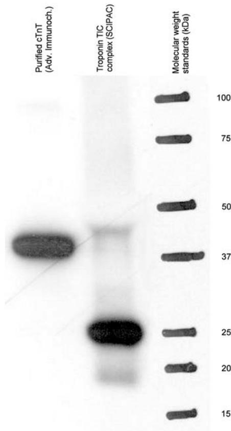
**Figure 3** Western blot of both cardiac troponin standards applied directly to SDS-PAGE. Detection was carried out with monoclonal anti-cTnT antibody 9G6 (epitope 1–60, HyTest). The intact protein is partly masked by the large amount of albumin present in the troponin TIC complex standard.
